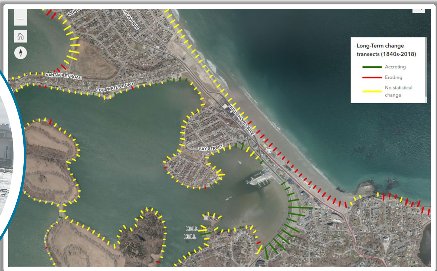
Low rates of long-term erosion at Nantasket Beach, Hull
